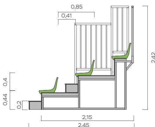
Important: the floor should not have more than 2% level variations, so that modules can be assembled together.
